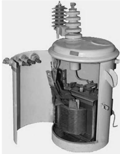
Figure 2.2 A self-protected distribution transformer typical of sizes 2 to 25 kVA, 7200:240/120 V. Only one high-voltage insulator and lightning arrester are needed because one side of the 7200-V line and one side of the primary are grounded.
