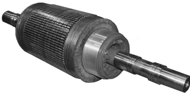
Figure 4.2 Armature of a dc motor. (Photo courtesy of Baldor Electric/ABB)
