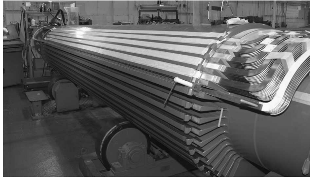
Figure 4.3 Field winding installation on the rotor of a 200-MW, 2-pole synchronous generator. (Photo courtesy of General Electric Company.)
